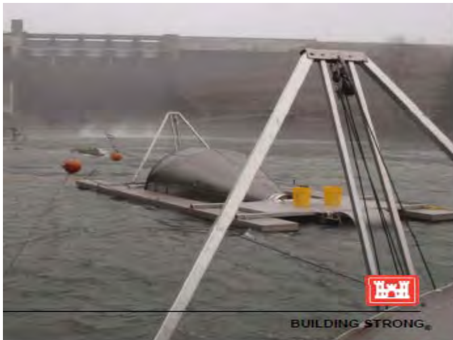
Figure 4-8. Example of Merwin Trap (reproduced from Raymond and Collins, 1975)
